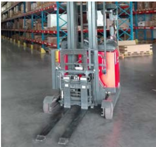
Fork Positioner With Load Stabilizer And Telescopic Forks T129 / 163 / 180BT
