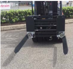
Fork Clamp With Turnable Forks T411DH
