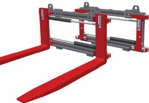
The range T160 with optimised visibility and residual capacity is fitted with valve block sideshift as standard. As valve block sideshift uses the rest stroke of the cylinder for the sideshift function the lateral shift is dependent on the fork position. Depending on the construction width of the attachment a lateral shift of up to  $\pm 300$  mm can be achieved. The possibility of the load being picked up off centre must be taken into account when calculating the residual capacity.
